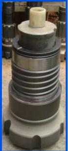
7. Screw the assembled *Drive Chuck* with *Bit* into the *Wear Sleeve* (Part No.1)
