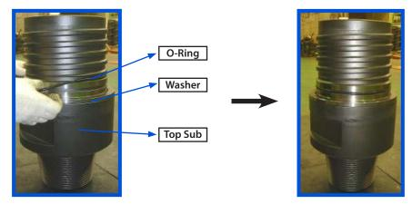
14. Screw the *Top Sub* (Part No.2) with above *Washer* & *O-ring* into top end of *Wear Sleeve* (Part No.1) tightly.
