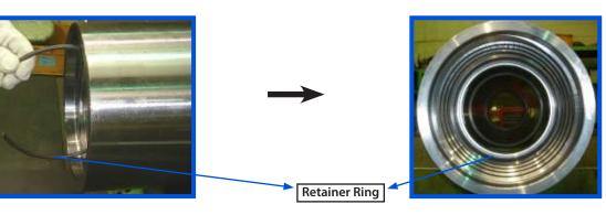
2. Insert *O-ring* (Part No.19) at the center groove of *Bit Retainer Ring* (Part No.18). And then insert *Bit Retainer Ring* (Part No.18) with *O-ring* into the *Wear Sleeve* (Part No.1)
