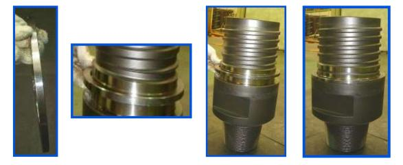
13.Insert the *O-Ring* (Part No. 3) on the groove of the *Top Sub* (Part No. 2) as shown.
