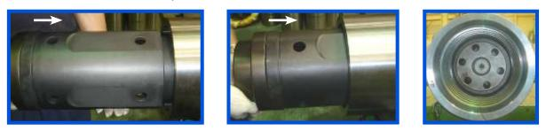
10. First put *Make-Up ring* (Part No. 6) and into Wear Sleeve (Part No. 1) tightly.
