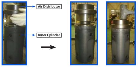
9. Put the assembled Inner Cylinder (Part No. 12) into the Wear Sleeve (Part No. 1).
