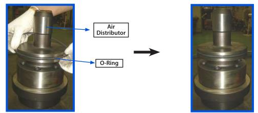
8. And then insert the *Air Distributor* (Part No. 10) with the *O-ring* above into the *Cylinder* (Part No. 12).
